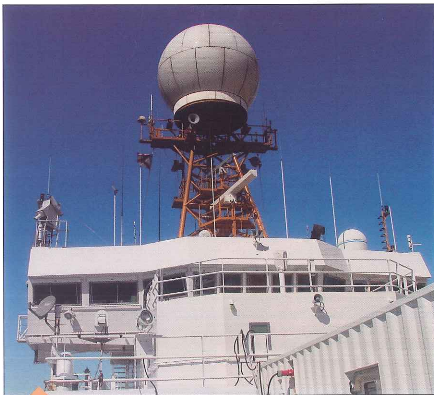
Photo 2. The University of Washington Calibrated IR In-situ Measurement System (CIRIMS) installed above the pilot house (left center) on the starboard side of the NOAA Ship Ronald H. Brown while in Pensacola, Florida during November 2003. Photo courtesy of Pablo Clemente-Colon.
